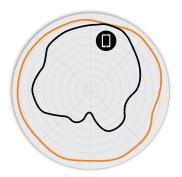
Figure 3. R650 5GHz Azimuth Antenna Patterns
