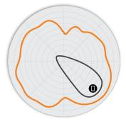
Figure 5. R650 5GHz Elevation Antenna Patterns
