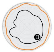
Figure 4. R650 2.4GHz Elevation Antenna Patterns
